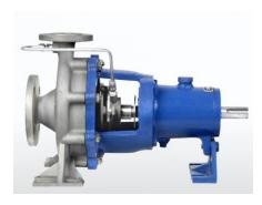
'JCPP' are in Back Pull-out Construction, Horizontal, Foot Mounted, Single Stage, End suction and Top Centerline Discharge, Confirming to DIN 24256 / ISO 2858, Standard and in general Confirming to API 610 as well.
