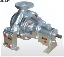
'JCLP' are in Back Pull-out Construction, Horizontal, Center line Mounted, Single Stage, End Suction and Top Centerline Discharge Suitable for Thermic Fluid & Hot oil also.
